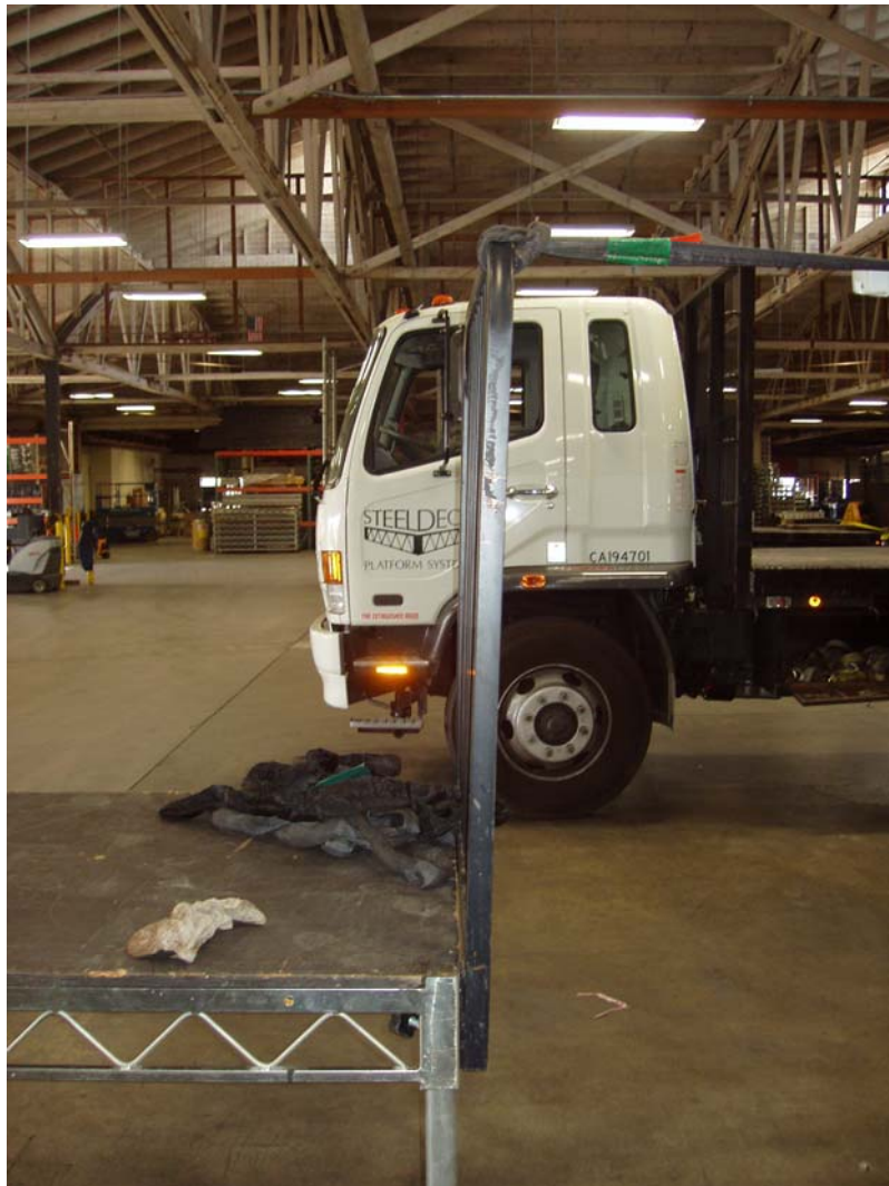
Figure 3-1 Elastic Deflection, Outboard Test #1 loaded to 207.1 lbs
