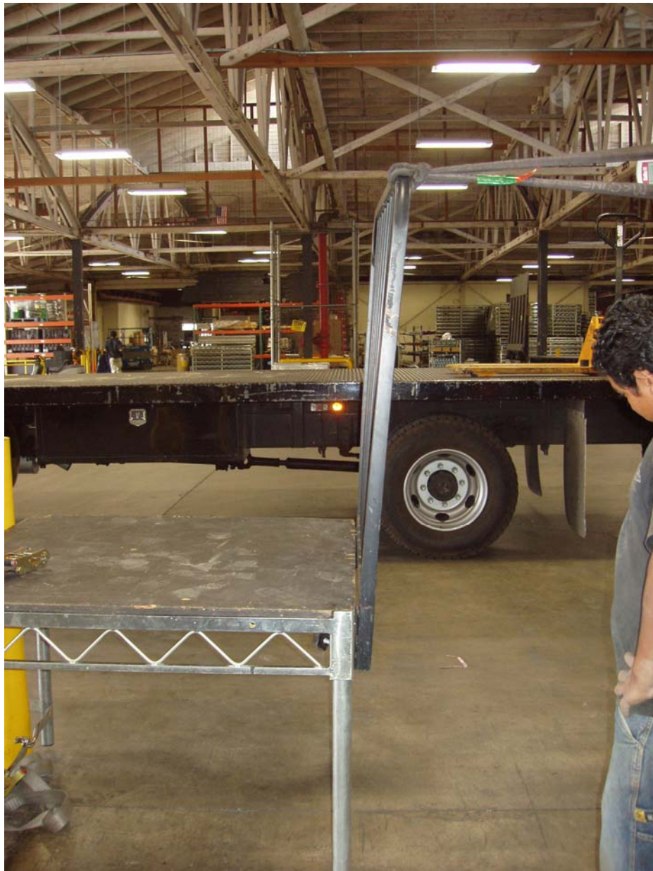
Figure 3-6 Elastic Deflection, Outboard Test #3 loaded to 382.1 lbs
