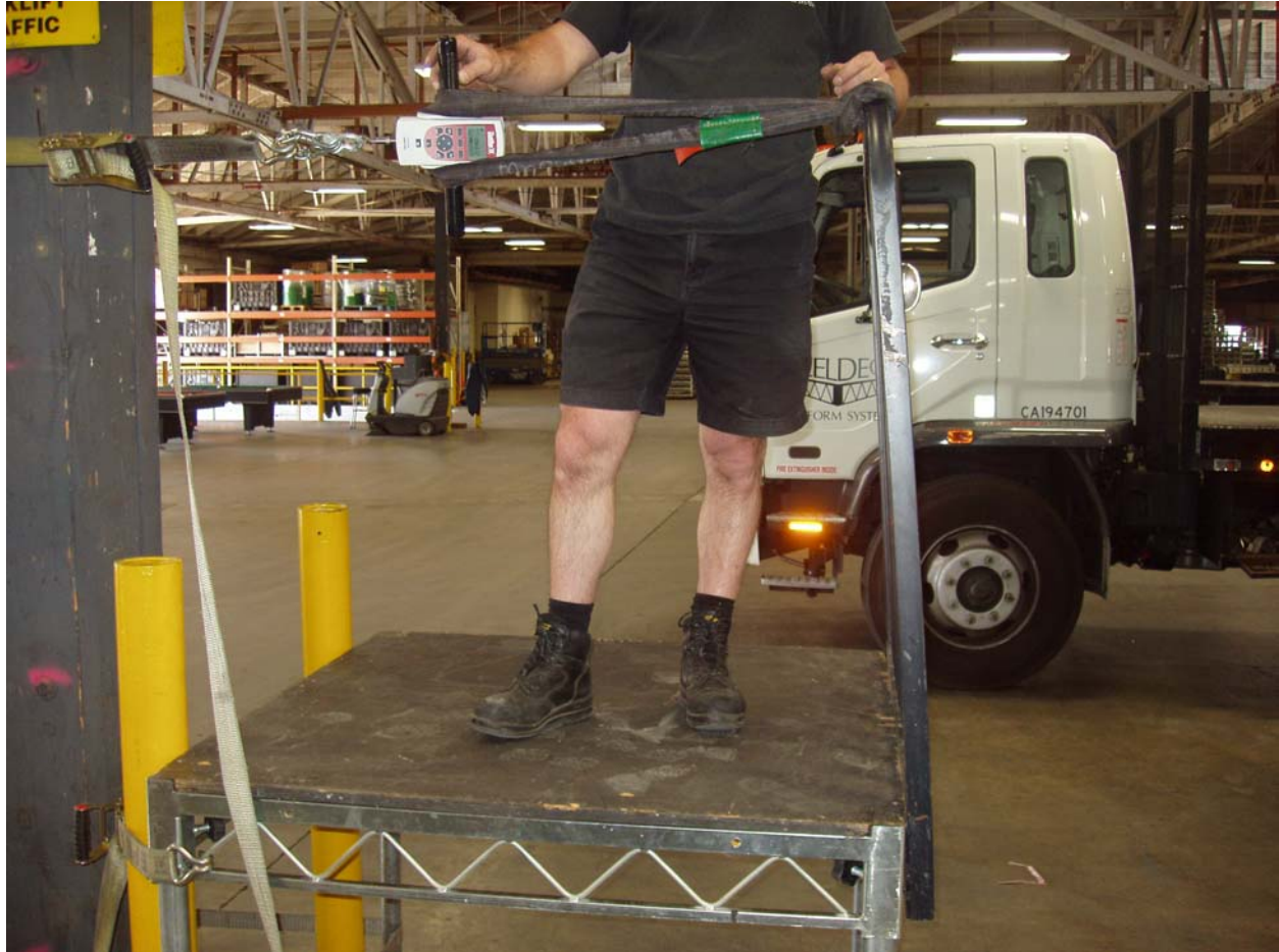
Figure 3-3 Elastic Deflection, Inboard Test #2 loaded to 214.4 lbs
