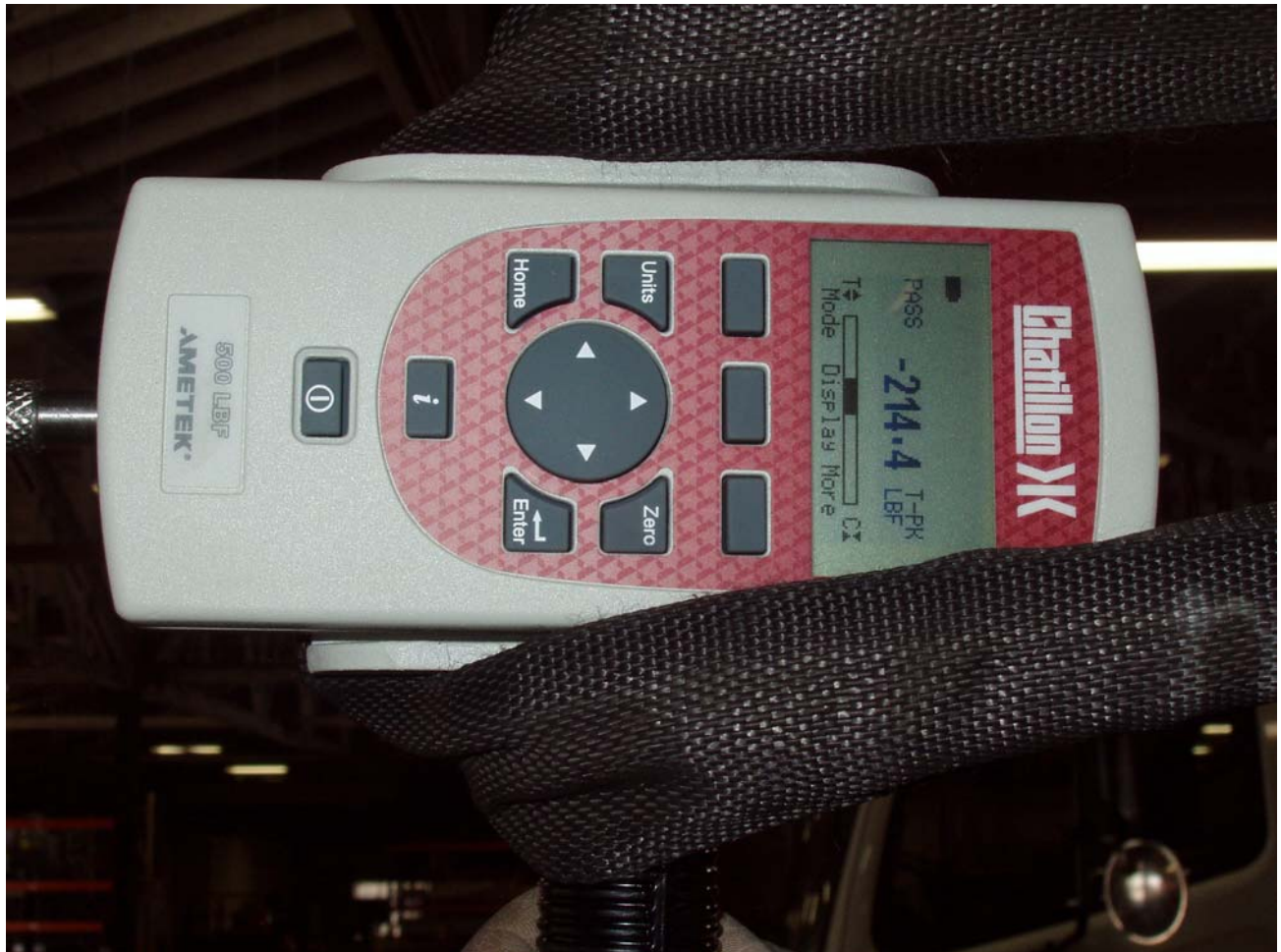
Figure 3-4 Inboard Test #2 loaded to 214.4 lbs
