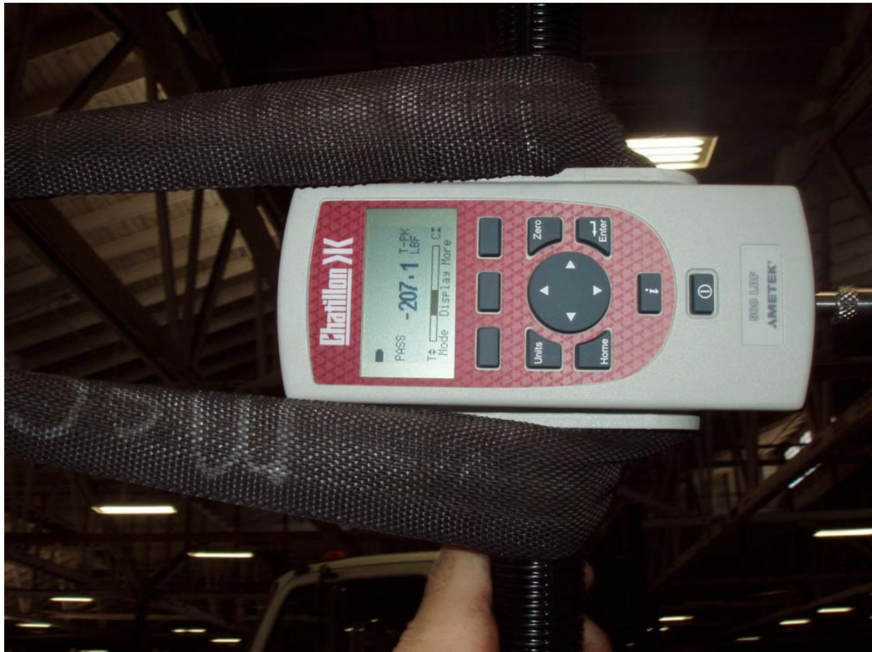
Figure 3-2 Outboard Test #1 loaded to 207.1 lbs
