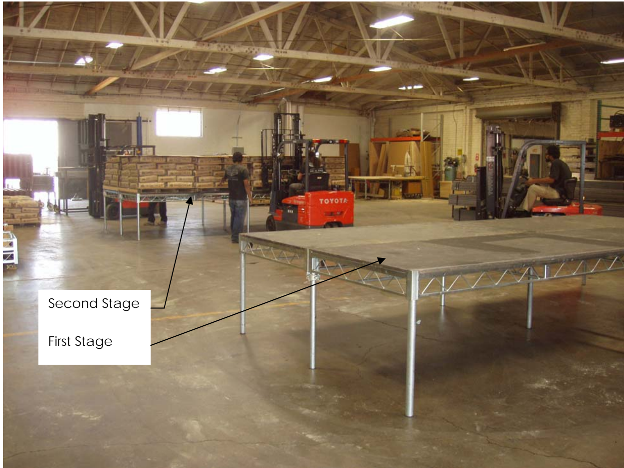
Figure 3-7 Load Step 4, 2 nd Stage loaded to 147.25 lbs/ft 2
