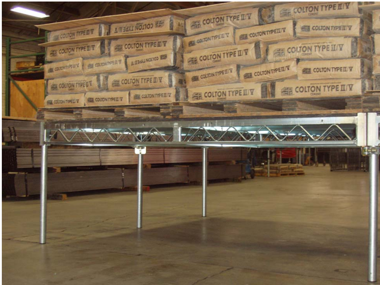
Figure 3-8 Load Step 4, 2 nd Stage loaded to 147.25 lbs/ft 2 , 3/16" Sag of 8' long beams
