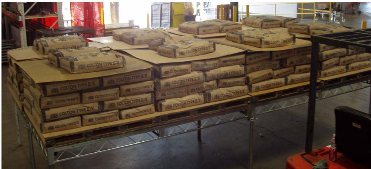
Figure 2-6 First Stage loaded to 135.5 lbs/ft 2
