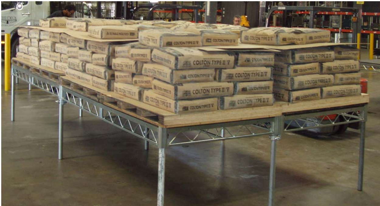
Figure 3-1 Load Step 1, 1 st Stage loaded to 135.5 lbs/ft 2
