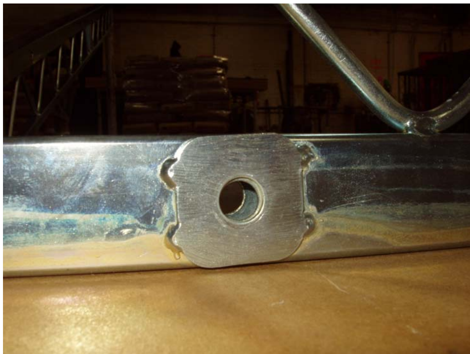
Figure 3-10 Load Step 15, 2 nd Stage, No distress of critical deck-to-deck bearing surfaces
