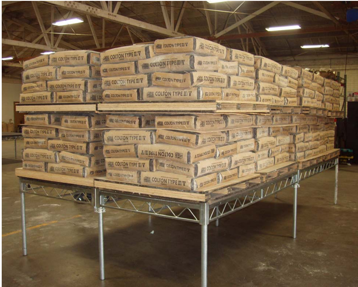
Figure 3-2 Load Step 2, 1 st Stage loaded to 271.0 lbs/ft 2
