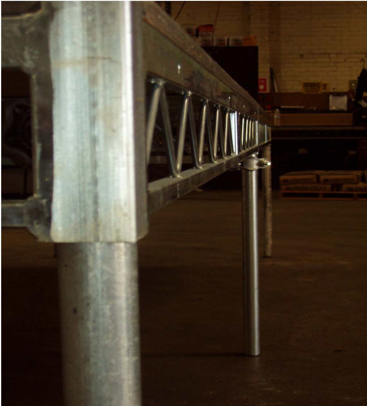
Figure 3-6 Load Step 3, 1 st Stage unloaded, Complete Elastic Recovery of side beams
